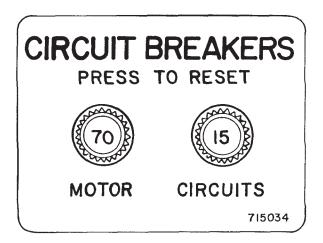
70 AMP circuit breaker protects pad drive motor from excessive overload conditions, i.e. excessive pad pressure, loaded pad.
